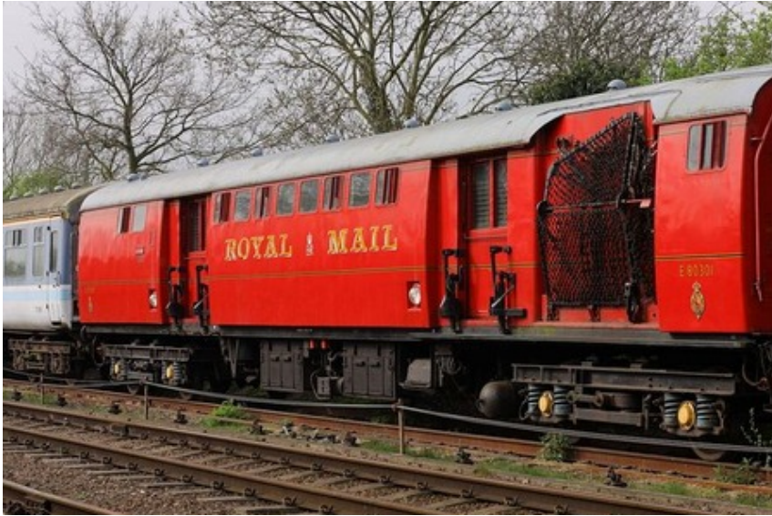
A Travelling Post Office coach with mail drop and catch mechanisms
